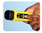
On/Off switch - press and release once to switch on, then once again to switch off.
